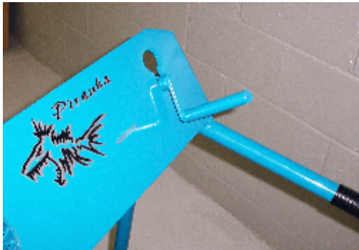
Fig. 4 Depth control in idle position
