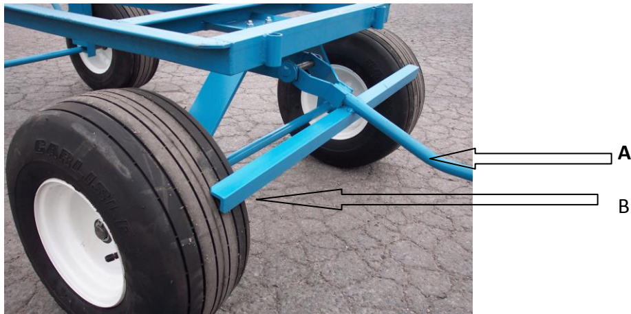
Fig. 2 Little Giant Controls A - Handle B - Brake
